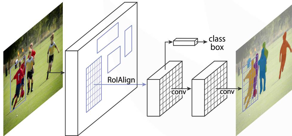
Figure 1: The **Mask R-CNN** framework for instance segmentation.
